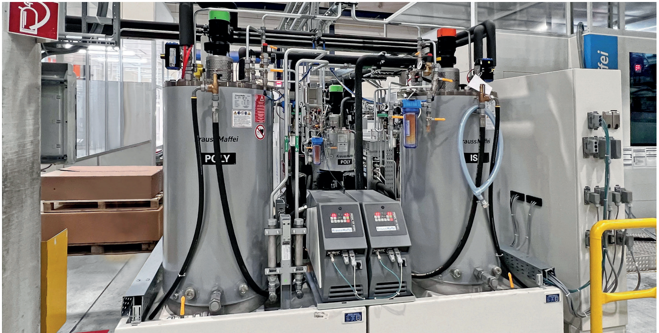
Fig. 3. KraussMaffei supplied both the MXW 1000 injection molding machine and the RimStar Flex mixing and metering machine. Two MK5-2K CCM mixing heads ensure high productivity of the ColorForm system. © KraussMaffei
