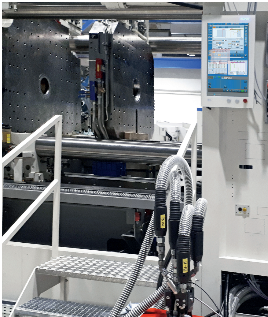
Fig. 2. The injection mold with swivel plate for the thermoplastic substrate makes the MXW 1000 from KraussMaffei particularly productive. © KraussMaffei
